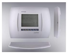
**IFS7002R** - The IFS7002R repeater panel allow vital information from the IFS7000 system to be communicated through points around the building, remote from the fire alarm control panels. Distributed at strategic points in a facility - such as nurse stations, floor landings, control rooms - valuable time can be saved when identifying the location of a fire and/or evacuating the building.
